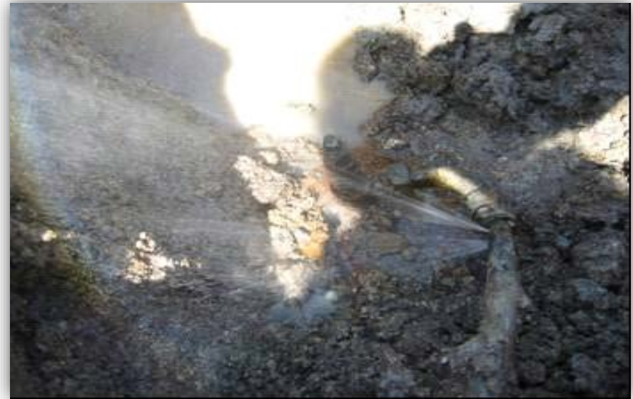
Customer service line leak
